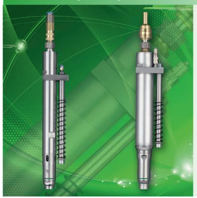
The SENSOMAT has been specially designed for screw joints where the screwdriving torque (forming torque) is close to or even higher than the shut-off torque due to high friction during assembly.
