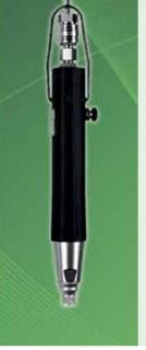
The MINIMAT-T is equipped with an adjustable finder/sensor sleeve which triggers motor shutoff at the required depth – consistently. The screwdriver is available in the straight or pistol grip form offering torque output options of 5-12 Nm.
